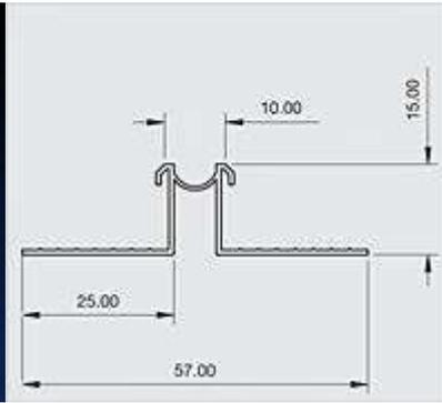
Locally manufactured from recycled plastic, Renderplas PVCu movement joint beads / expansion joints are designed for areas of render over 20 square metres and should be specified every 4-6 metres, over structural movement joints and changes of background. Discreet but strong, all beading gives a perfect finish to through colour render and is equally suitable for sand and cement
